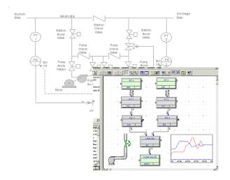
Automatic report generation includes tabular reports containing all blocks in the system, their internal parameters, and all connections, as well as graphical reports showing the database diagram exactly as it is drawn. Once the database has been defined and saved, it is downloaded to individual MODCELL Multiloop Processors or MOD 30ML Multiloop Controllers using either the Extended Modbus or ICN OPC Server.
